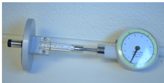
Figure 1: Picture of the Tissue compliance meter.
